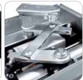
Detail of the motor-pump and jack
