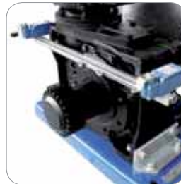
Drive gear and mechanical limit switches
